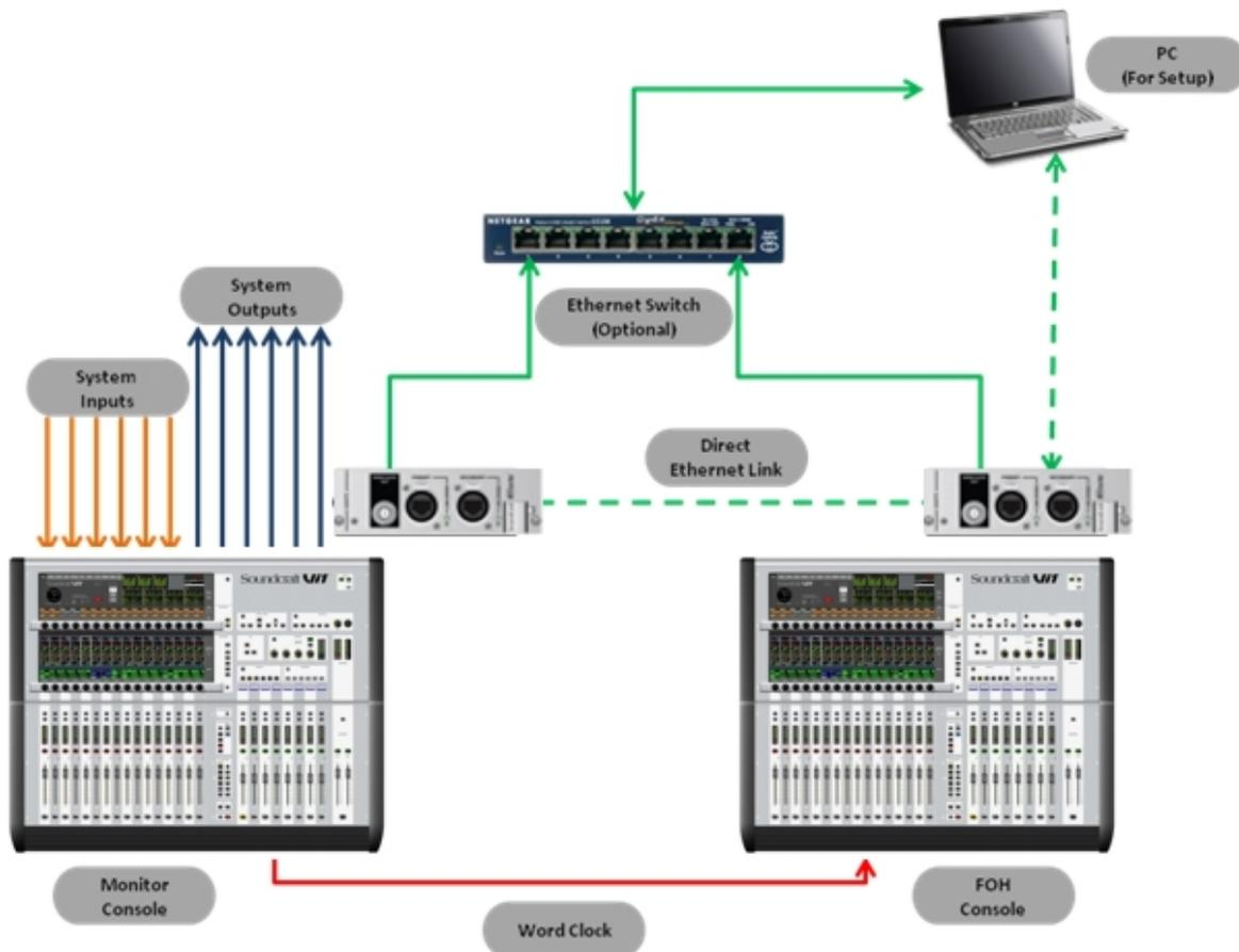
Audio inputs are sent to the monitor console, these can be connected directly to the console or via a stagebox attached via a MADI card to the monitor console.
