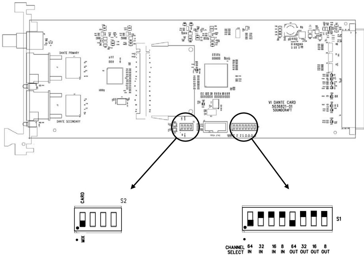
Note! Switches point **down** to select channel count – ignore the 'ON' legend on switch body!
