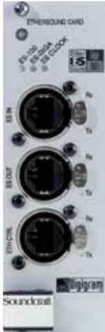
The Digigram EtherSound card allows up to 128 channels of audio (64 inputs/64 outputs) to be connected to the rack via a single Cat5 connection. A second Cat5 connection allows daisy chaining or full redundancy capability, ensuring the network remains uninterrupted should a cable be broken.
