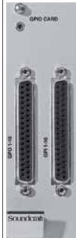
For general-purpose switching applications requiring total electrical isolation, this card provides 16 electrically isolated opto-coupler inputs with integrated current sink (5...24 VDC) and 16 electrically isolated outputs using SPST relay contacts. 5 VDC supply pins are available. Inputs
