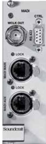
Two types of MADI card are available, both offering 64 channels of audio on dual redundant cables. The Cat 5 version offers cost-effective connections to a Soundcraft Stagebox using Cat 5 cable terminated in robust Ethercon connectors. Distances of up to 120m are possible using approved
